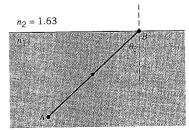
light strikes the interface at the critical angle of  $\theta_c = 48.1^{\circ}$ . How much time does it take for the light to travel from A to B?
