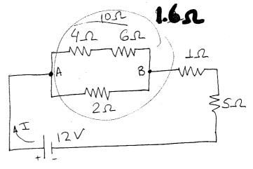
(a) (10 points) Find the equivalent resistance of the circuit.
