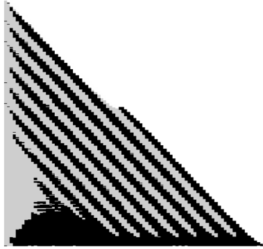
Fig. 2. Resulting morphology of the numerical integration of the continuum equations. Large grains are black and small grains are gray. The parameters used are \tan(\theta_{11}) = 1 , \tan(\theta_{22}) = 1.1 , \tan(\theta_{12}) = 1.4 , \tan(\theta_{21}) = 0.7 , \gamma = 0.8 , and v_1 = v_2 = 1 .
